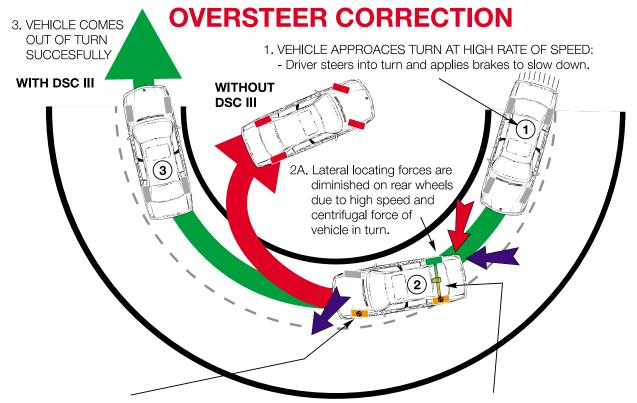
2D. The torque reduction and rear brake regulation should stabilize the vehicle at this point. If not the left front wheel has a high degree of lateral locating force and is momentarily regulated.
